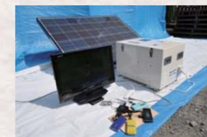
One form of aid was a solar power system for disaster relief that combined solar cells and storage batteries. Produced in collaboration with Shin-Kobe Electric Machinery Co., Ltd., these systems were donated to emergency shelters. The stored power generated from sunlight was used for purposes such as charging mobile phones and watching television.
