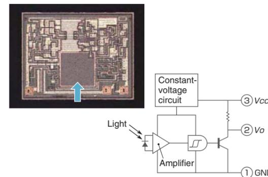
The square in the center (arrow) is the photodiode (light-receiving component); the area around it is occupied by signal-processing circuitry (IC).
