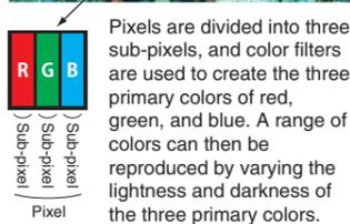
Pixels are divided into three sub-pixels, and color filters are used to create the three primary colors of red, green, and blue. A range of colors can then be reproduced by varying the lightness and darkness of the three primary colors.
