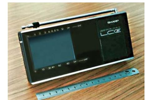
Prototype 3.2-inch TFT color LCD TV (1985)
