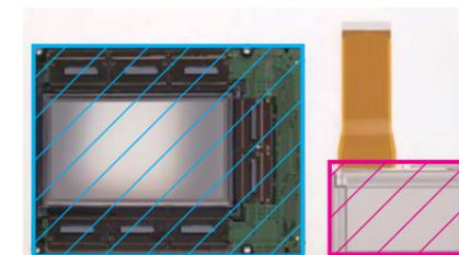
A System LCD (right) has fewer peripheral components and requires a smaller mounting area (shown with diagonal lines) than conventional LCDs. The photographs provide a comparison for LCDs used in projectors.
