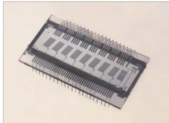
Prototype of LCD used for electronic calculators (1972)
