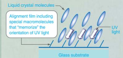
Once the orientation of the alignment film is determined by irradiating the substrate with ultraviolet (UV) light during the manufacturing process, the liquid crystal molecules are aligned in the same direction.
