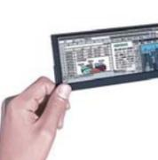
High-reflective Super Mobile LCD for the outdoor display of bright color images without the need for a backlight
