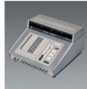
World's first all-transistor-diode desktop calculator
