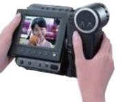
LCD ViewCam, which allowed users to shoot video while watching an LCD viewfinder and enabled instant playback of just-taken footage
