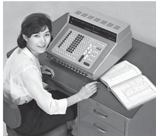
The CS-10A, the world's first all-transistor diode electronic desktop calculator
