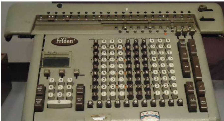
One of the most advanced electromechanical calculators Friden Model SRQ (~1962)
