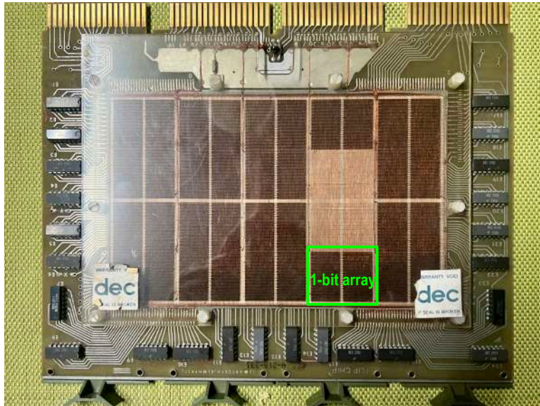
Part of the magnetic core memory of the Digital PDP-11 (1973)
