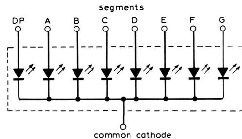
Fig. 6. The circuit of one of the gallium arsenide indicators showing how the eight light-emitting diodes are connected.
