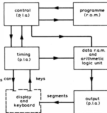
Fig. 3. Block diagram of the calculator integrated circuit.
