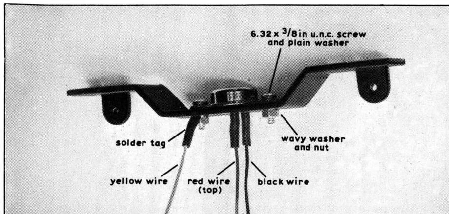
( ) Solder red wires to the terminals indicated in the photograph. Place the assembly on one side.
