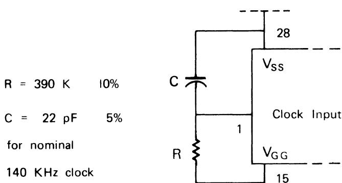
The oscillator waveform appears as a "sawtooth" voltage variation swinging between  $V_{SS}$  and  $V_{GG}$ /2.
