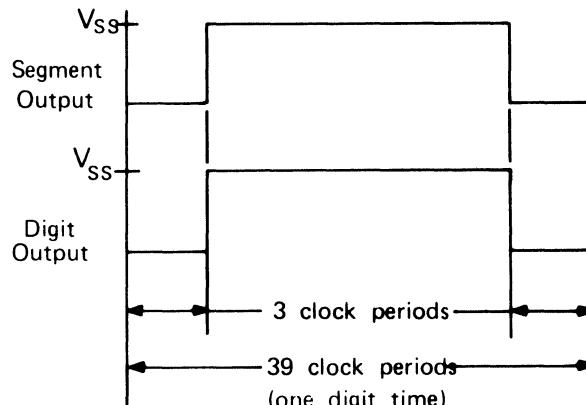
Note: Segment and digit outputs are turned on to  $V_{SS}$  for a displayed segment.
