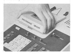
Remove the upper panel, take off the instruction tag from the ribbon, and set the ribbon correctly.
